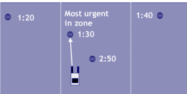
Figure 4. WMS assigns most urgent task within the zone.
